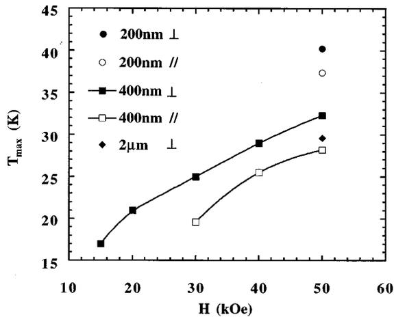
FIG. 3. The dependence of resistance maximum  $T_{\max}$  on magnetic field for various wire diameters, where solid and open symbols stand for transverse ( $\perp$ ) and longitudinal ( $\parallel$ ) field geometry, respectively.
