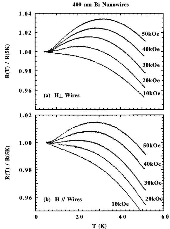
FIG. 2. Temperature dependence of resistance (normalized to the value at 5 K) of the 400-nm Bi wires showing resistance maximum at  $T_{\text{max}}$  for various values of (a) transverse and (b) longitudinal magnetic field.
